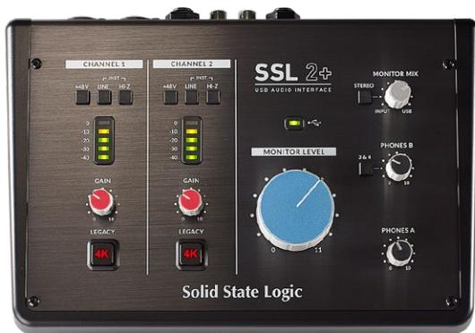
rear panel output jacks. The Monitor Mix blend control balances between "Input"—the live audio coming in and "USB" or the audio returning from the DAW.
